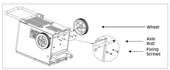
3. Once the wheels have been installed, place the machine in the upright position.
